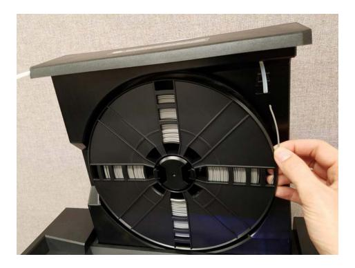
**7.** Now, place the end of the filament into one of the four sets of holes on the outside of the filament to prevent unwinding. First use the closest hole of the set and then the furthest as shown in the photo below.
