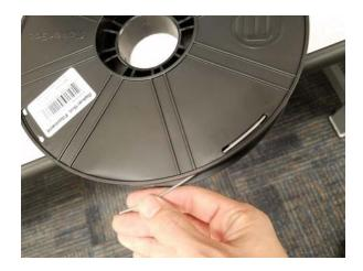
**8.** We are now ready to place the new spool of filament into the filament drawer. If the drawer is closed refer to **Step 4** on how to open. Be sure to align the spool so that the filament feeds out clockwise and into the guide tube (the white tube).
