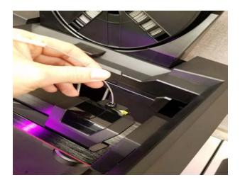
**10.** On the front control panel select **Filament > Load Filament**. The printer may need to heat back up again. Once the printer is ready the onboard display will prompt you to insert the filament into the top of the extruder. Follow the on screen display for instructions.
