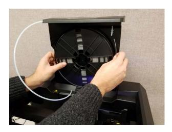
**9.** Trim the end of the filament (if needed) so that there is a clean edge. Begin feeding the filament into the guide tube. Continue feeding until an inch or so of filament is sticking out of the end of the guide tube nearest the extruder (as shown).
