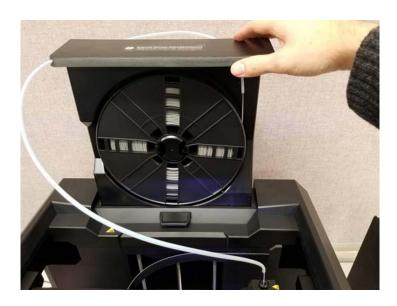
**6.** Now, unload the filament by rotation filament spool clockwise. Be sure to grab ahold of the end of the filament (as seen below). While holding onto the spool and the end of the filament, gently pull the spool towards you to remove from the machine.
